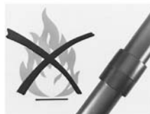
No open flames when cementing. No smoking.
