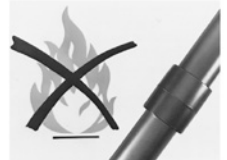
No open flames when cementing. No smoking.
